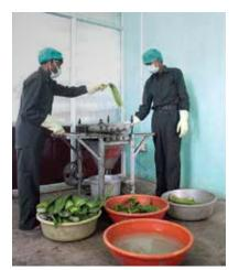
Aloe Vera gel is extracted from a crushing machine.
