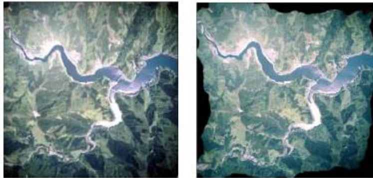
Figure 1 Aerial photo (left) and digital ortho (right)
