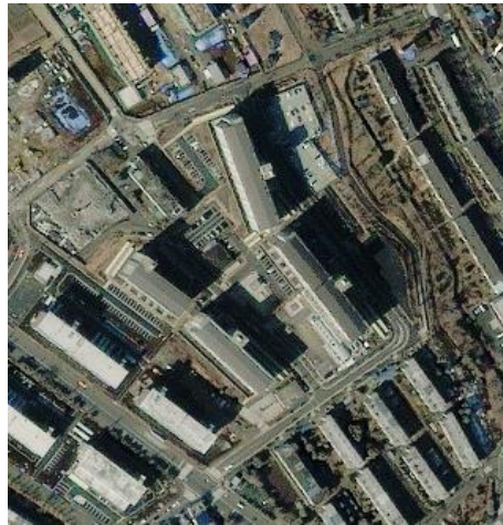
Slanting of buildings due to relative elevation differences (IKONOS satellite image example)
