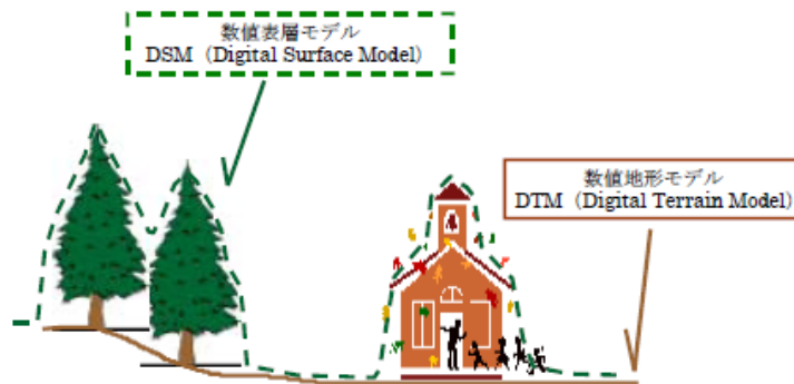
Figure 4 DTM and DSM
