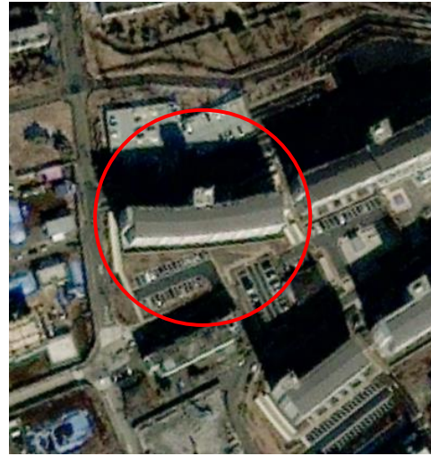
Local distortion of buildings (IKONOS satellite image example)
