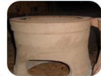
Solution 2 : Strengthen by more red earth and less clay.
