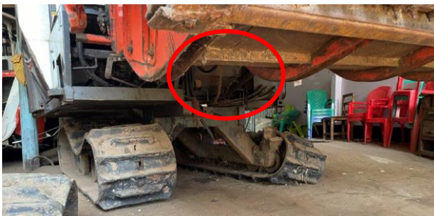
A combine harvester whose transmission could not be repaired, and hence, it was out of operation
