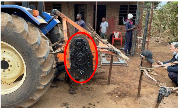
Repairing the rotary as the drive gear was missing
