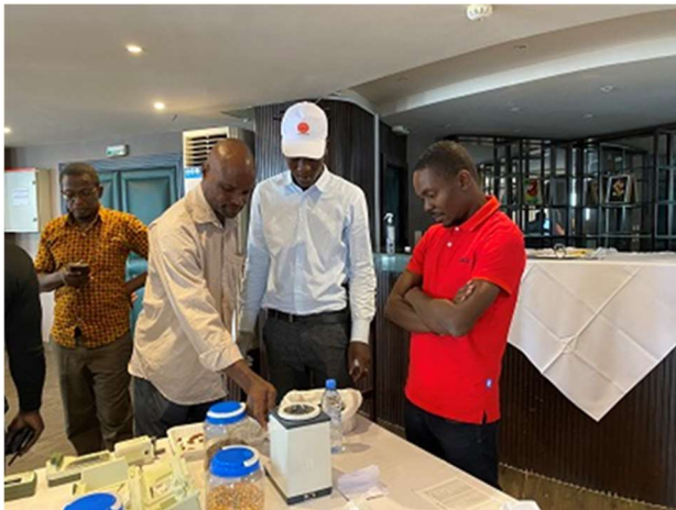
A participant from a cacao production and processing cooperative (Left) measuring the moisture content of cacao using a Kett instrument.
